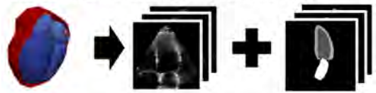
Fig. 1. Using anatomical models as high quality ground truth annotations, we propose a pipeline to generate large synthetic datasets for training convolutional neural networks.
